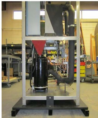
Figure 1 - Example of Red Shipping Bracket
