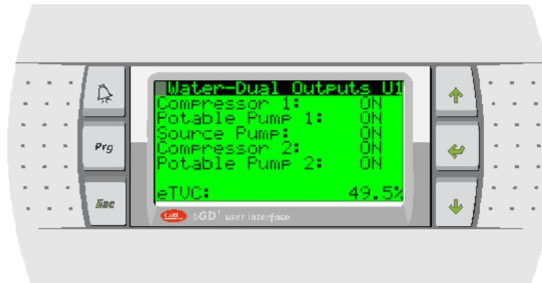
Below is the general appearance of the first I/O screen of an air-source heat pump. (Though the actual analog inputs may have different nominal values from those depicted.)
