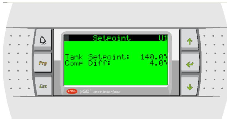
The Setpoint menu will display the following for a two-compressor unit with aquastat set to “Internal”:
