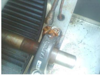
Figure 10 - Excessive Lubrication Damage
