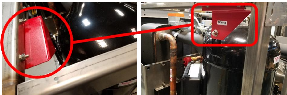
Figure 2: Shipping bracket to be removed before operation.
